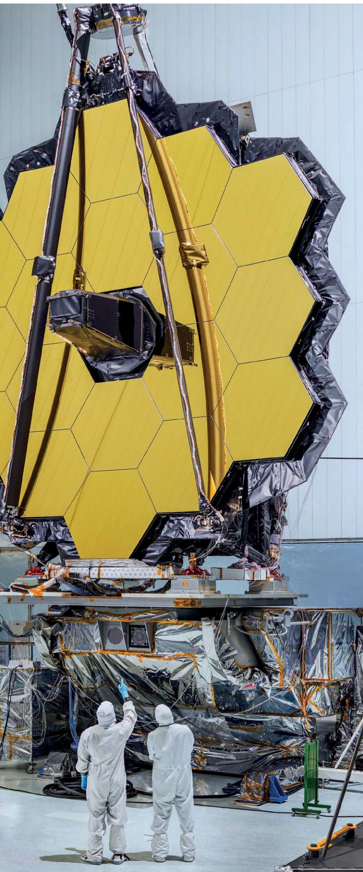
The primary mirror of NASA's James Webb Space Telescope consisting of eighteen hexagonal mirrors standing in the massive clean room of NASA's Goddard Space Flight Center in Greenbelt, Maryland. NASA MEDIA
